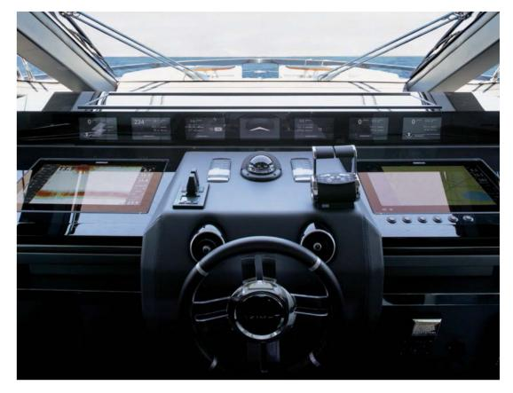
The bridge was produced in partnership with Simrad-Naviop and has a single ultra-wide screen displaying key monitoring and navigation information, a mix of video sources and clusters of content. Accessing this information is easy with a choice of commanders or two touch screens duplicated by a pair of physical joggers for extra redundancy and safety.
