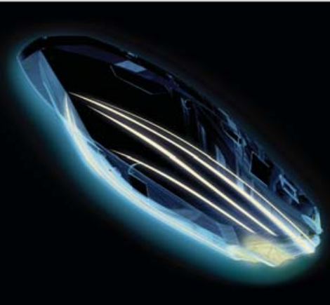
Hard-chine planing hull with variable deadrise (Flybridge and Atlantis Collections)
