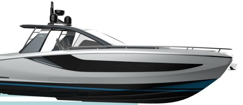
The combination of deep 'V', steps and ventilated aft tunnel add up to being the most efficient high speed rough water hull form developed today.
